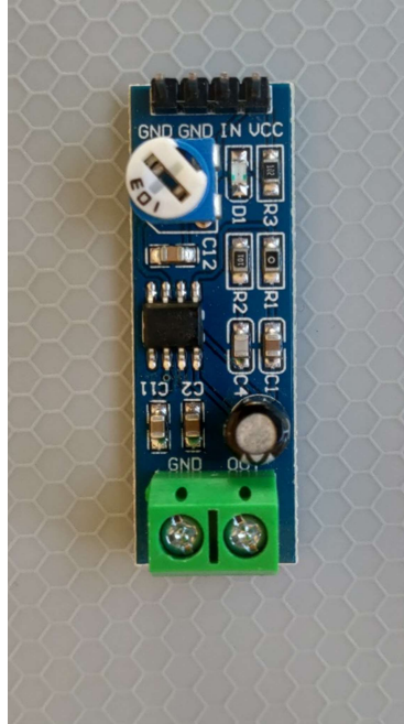
Fig. 5 – Picture of amplifier with the correct position for volume dial
